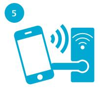
After ensuring that the Bluetooth is enabled, the guest simply holds the smartphone to the door lock, waits for the solid green light and enters the room.
